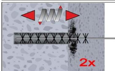
2b. Brush the bore hole minimum 2x with brush RB according to Table B4 over the entire embedment depth in a twisting motion. (If necessary, a brush extension RBL shall be used.)
