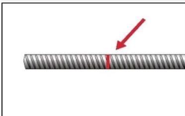
4. Mark embedment depth on the reinforcing bar.
