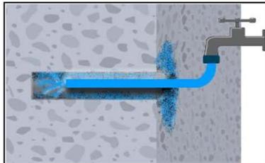
2c. Flushing again with water until clear water comes out.
