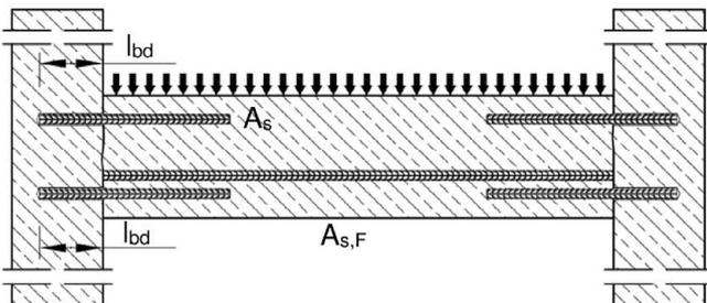
**Figure A4:** Rebar connection for components stressed primarily in compression. The rebars are stressed in compression
