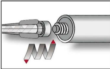
3. Screw on static-mixing nozzle PM-19E, and load the cartridge into an appropriate dispensing tool.
