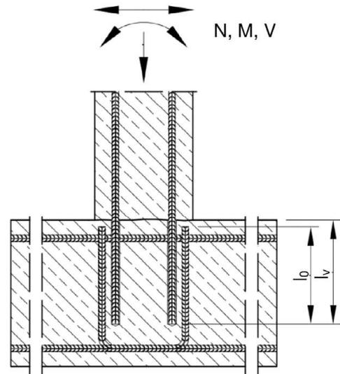
**Figure A3:** End anchoring of slabs or beams (e.g. designed as simply supported)
