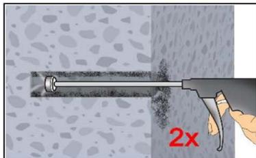
2d. Blow the bore hole clean minimum 2x with compressed air (min. 6 bar) (Annex B 6) over the entire embedment depth until return air stream is free of noticeable dust. (If necessary, an extension shall be used.)
