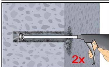
2f. Finally blow the bore hole clean minimum 2x with compressed air (min. 6 bar) (Annex B 6) over the entire embedment depth until return air stream is free of noticeable dust. (If necessary, an extension shall be used.)
