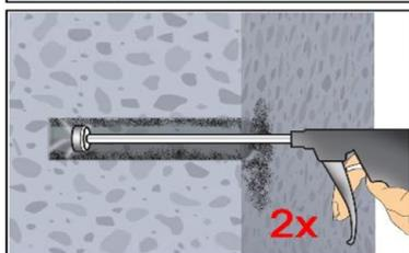
2c. Finally blow the bore hole clean minimum 2x with compressed air (min. 6 bar) (Annex B 6) over the entire embedment depth until return air stream is free of noticeable dust. (If necessary, an extension shall be used.)
