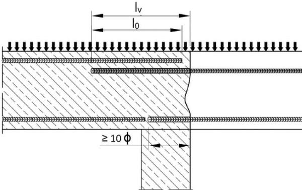
**Figure A2:** Overlapping joint at a foundation of a wall or column where the rebars are stressed in tension
