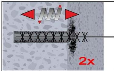
2b. Brush the bore hole minimum 2x with brush RB according to Table B4 over the entire embedment depth in a twisting motion. (If necessary, a brush extension RBL shall be used.)
