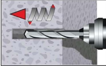
**1a. Hammer drilling (HD) / Compressed air drilling (CD)**
