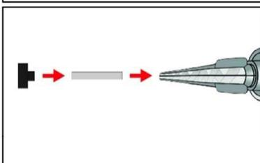
7. Piston plugs VS and mixer nozzle extensions VL shall be used according to Table B4 or B5.
