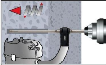
**1b. Hollow drill bit system (HDB) (see Annex B 6)**
