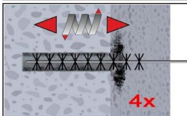
2b. Brush the bore hole minimum 4x with brush RB according to Table B4 over the entire embedment depth in a twisting motion (if necessary, use a brush extension RBL).
