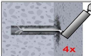
2c. Finally blow the bore hole clean minimum 4x from the bottom or back by hand pump (Annex B 6).
