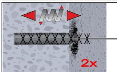
2e. Brush the bore hole minimum 2x with brush RB according to Table B4 over the entire embedment depth in a twisting motion. (If necessary, a brush extension RBL shall be used.)
