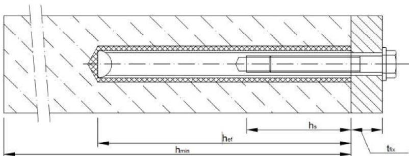
$t_{\text{fix}}$  = thickness of fixture
