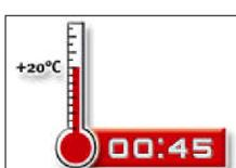
10. Allow the adhesive to cure to the specified time prior to applying any load or torque. Do not move or load the anchor until it is fully cured (attend Annex B 6).
