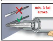
5. Prior to dispensing into the anchor hole, squeeze out separately a minimum of three full strokes and discard non-uniformly mixed adhesive components until the mortar shows a consistent grey colour. For foil tube cartridges it must be discarded a minimum of six full strokes.
