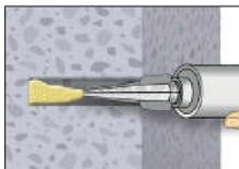
6. Starting from the bottom or back of the cleaned anchor hole, fill the hole up to approximately two-thirds with adhesive. Slowly withdraw the static mixing nozzle as the hole fills to avoid creating air pockets. If the bottom or back of the anchor hole is not reached, an appropriate extension nozzle must be used. Observe the gel-/ working times given in Annex B 6.
