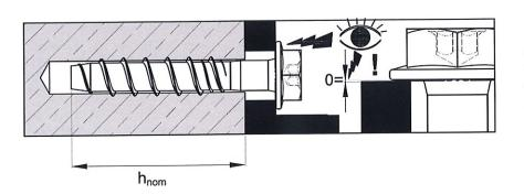
Ensure that the screw anchor head fully rests without any gap on the fixture and is not damaged
